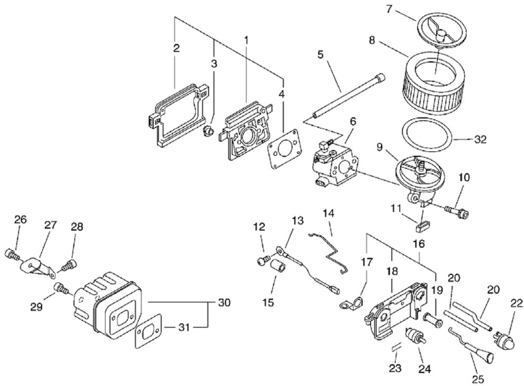
CS-450(30), -1--1, Air Cleaner, Carburetor, Muffler
