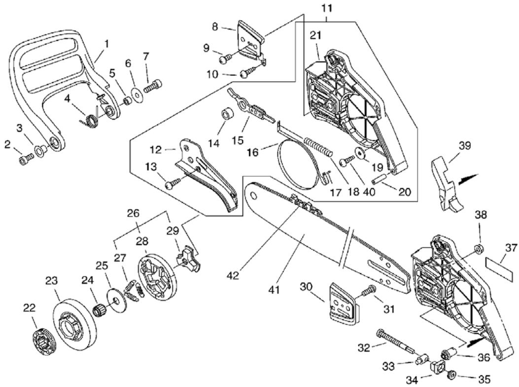
CS-450(30), -1--1, Clutch, Sprocket
