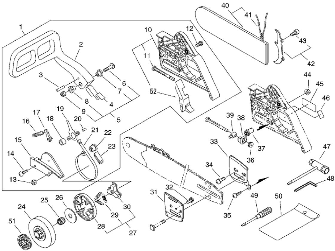
CS-680(30), -1--1, Clutch,Sprocket,Brake handle,Tool
