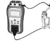
Test circuits for Insulation resistance measurement
