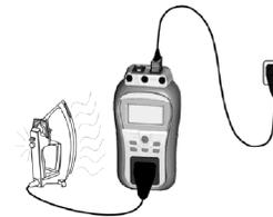
Test circuits for Substitute leakage current measurement
