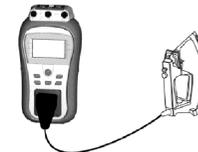
Test circuits for touch leakage current measurement
