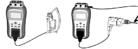
Test circuit for differential leakage current measurement
